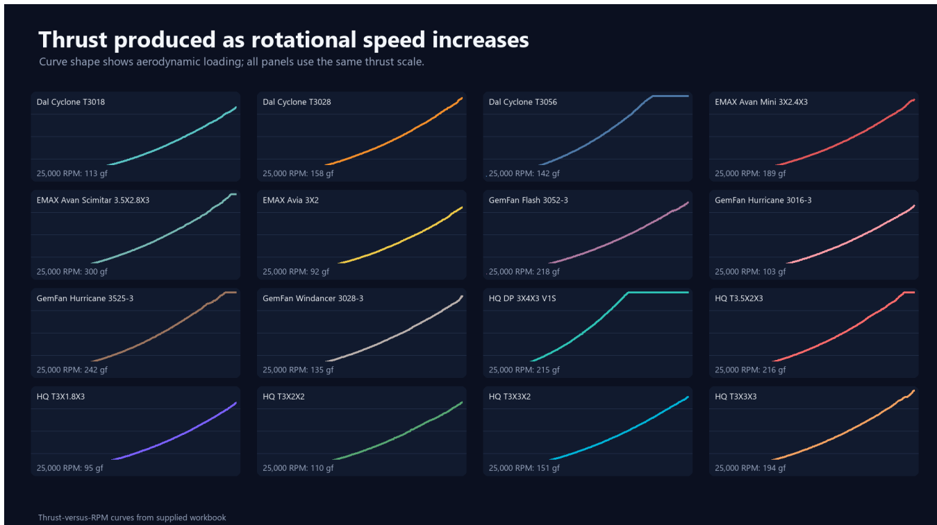
Figure 4. Thrust versus rotational speed. All panels use a common thrust scale.
