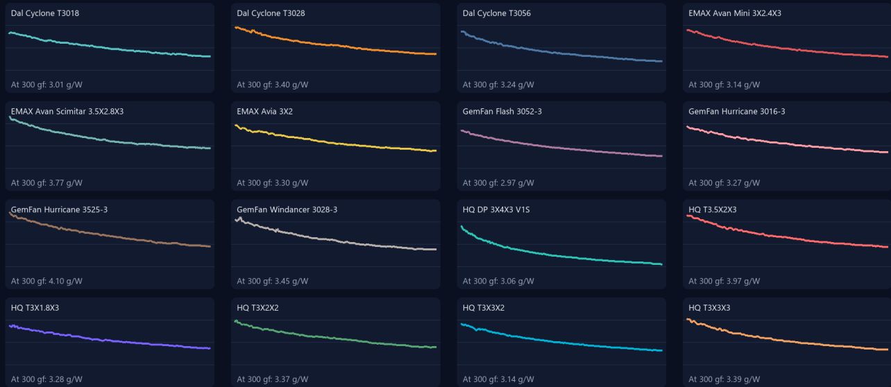
Figure 5. Mechanical efficiency across thrust. Higher curves indicate more thrust per shaft watt.
