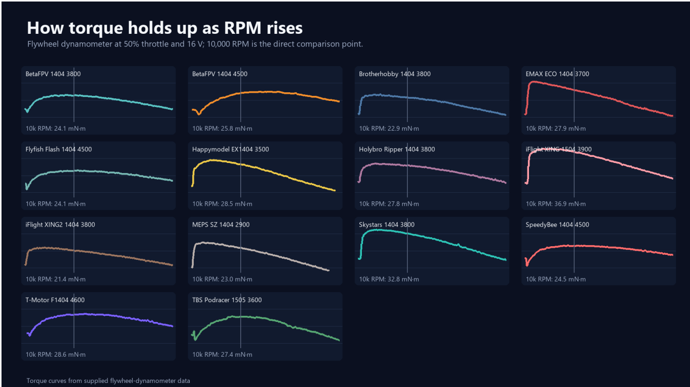
Figure 5 Flywheel-dynamometer torque curves from approximately 5,000 to 20,000 RPM
